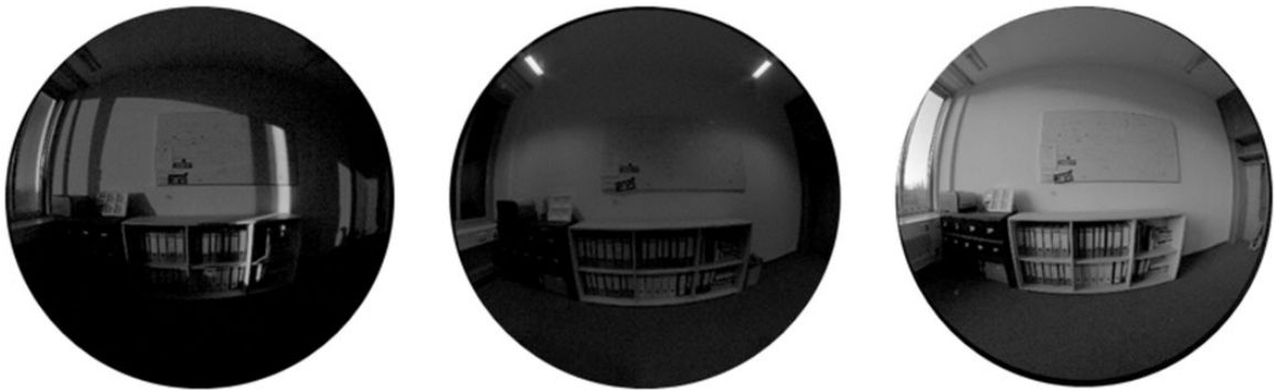
Figure 6 Spatial light distribution due to daylight (left, right) and electric lighting (middle).
