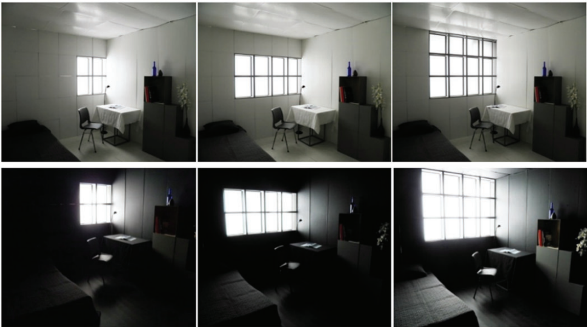
Figure 7 Spatial light levels due to daylight.
