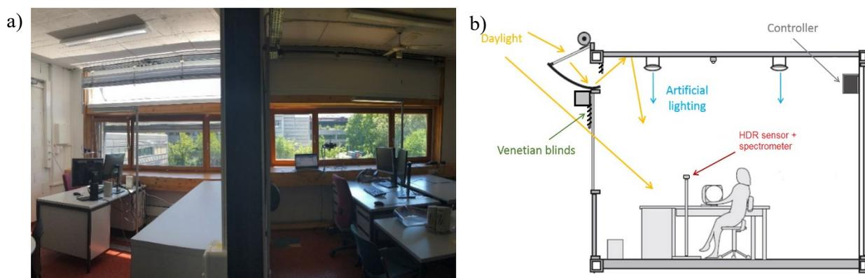
**Figure 1.** (a) View of the two office rooms. On the left side: test room, with ADS and automated control of venetian blinds and electric lighting; on the right side: reference room, with ADS closed and manual control of blind and lighting. (b) Cross-section scheme of an office room.
