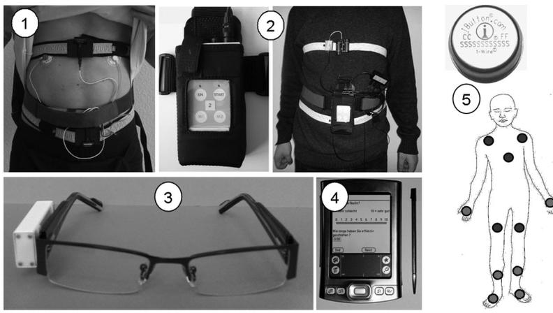
Figure 2. Ambulatory monitoring devices: 1) ClockWatcher: ECG, respiration, 3-dimensional acceleration, core body temperature; 2) Varioport: same channels as ClockWatcher; 3) Light sensor: ambient light, temperature, and 3-dimensional acceleration (for compliance check); 4) Palm computer: electronic diary (E-Diary); and 5) iButton: position of skin temperature measurements.
