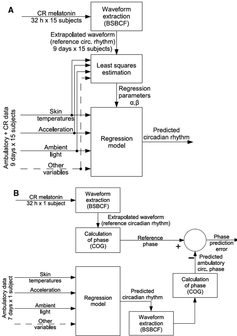
Figure 3. Modeling approach: (A) identification of a prediction model with ambulatory and CR data, and (B) validation of a prediction model with ambulatory data and CR melatonin for comparison of the predicted phase with the reference phase. The final structure of the regression model included only skin temperatures, motion acceleration, and irradiance for blue light as the input variables with their respective lags.
